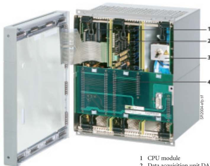
Fig. 13/71 Layout of a SIMEAS R
