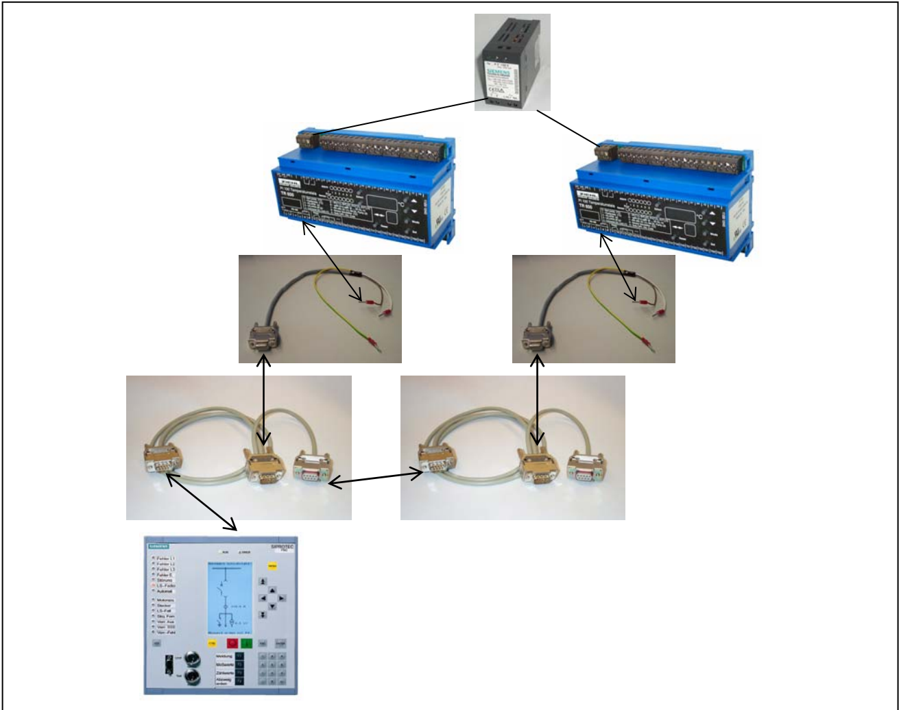
Picture 11: Connection with 2 RTD boxes
