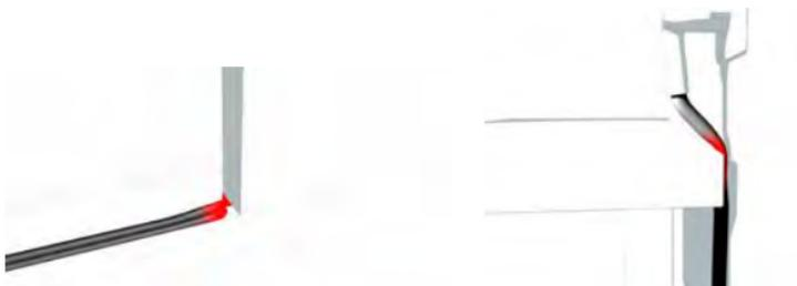
Figure 10: Crushed cable
