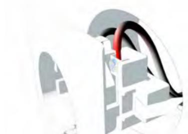
h) Conductors damaged by claw fasteners
