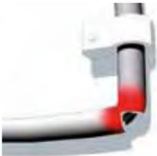
*Figure 9: Too tight a bending radius*
